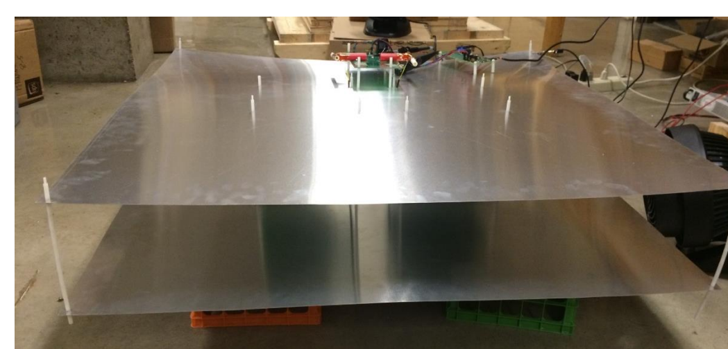
Testing under realistic vehicle environment – metal shields emulate the vehicle chassis and road
