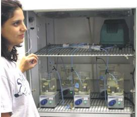
Monica Torres-Ruiz demonstrates the successful design for the flow-simulating caddisfly beakers with stir plates and an incubator.
